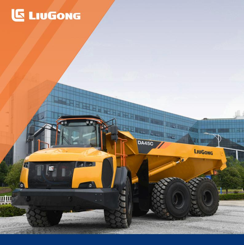
Max. Gross Machine Weight74,000 kgNet Machine Weight33,000 kgPayload41,000 kgEngineQSM15Rated Power563 kW (755 hp / 765 ps) @ 2,100 rpmStruck Capacity20.2 m³Heaped Capacity (SAE 2:1)25.6 m³
