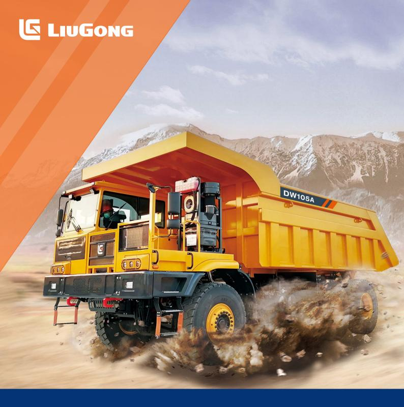
Max. Gross Machine Weight105,000 kgNet Machine Weight36,000 kgPayload70,000 kgEngineYC6K520Rated Power382 kW (512 hp / 519 ps) @ 1,900 rpmStruck Capacity36 m³Heaped Capacity (SAE 2:1)43 m³
